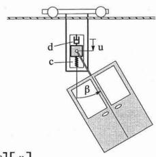
$$\begin{bmatrix} 1 & 0 \\ 0 & 1 \end{bmatrix} \begin{bmatrix} \ddot{\mathbf{u}} \\ \ddot{\boldsymbol{\beta}} \end{bmatrix} + \begin{bmatrix} d & 0 \\ 0 & 0 \end{bmatrix} \begin{bmatrix} \dot{\mathbf{u}} \\ \dot{\boldsymbol{\beta}} \end{bmatrix} + \begin{bmatrix} c & 0 \\ 0 & 5 \end{bmatrix} \begin{bmatrix} \mathbf{u} \\ \boldsymbol{\beta} \end{bmatrix} = \mathbf{h}(t) .$$
