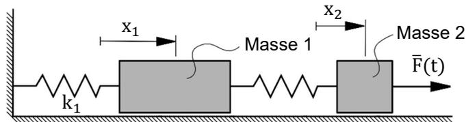
$$\underbrace{\begin{bmatrix} 4 & 0 \\ 0 & 2 \end{bmatrix}}_{\mathbf{M}} \cdot \ddot{\mathbf{y}} + \underbrace{\begin{bmatrix} k_1 + 4 & -4 \\ -4 & 4 \end{bmatrix}}_{\mathbf{Q}} \cdot \mathbf{y} = \begin{bmatrix} 0 \\ 1 \end{bmatrix} \bar{F}(t).$$
